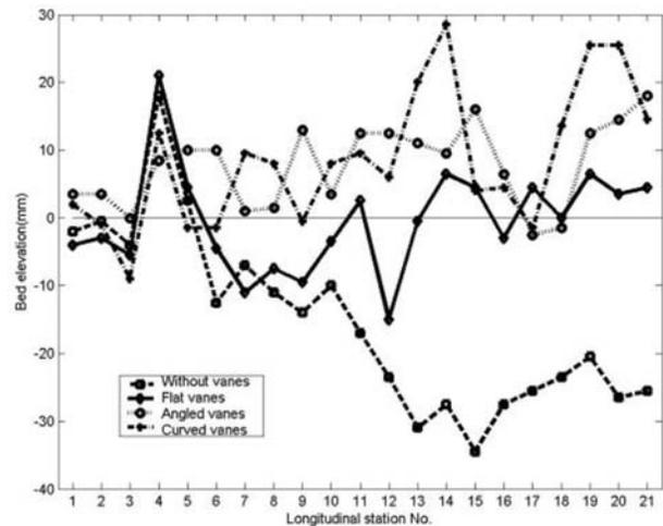
**Fig. 10.** Longitudinal bed profiles 3- vanes in a row in parallel pattern on 90° bend
