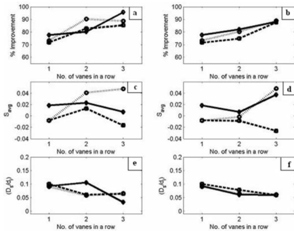
**Fig. 12.** Erosion indices of three shapes of vanes (—●— flat, —◇— curved and ....o.... angled) at different arrays of parallel (a,c,& e) and zigzag (b, d & f) pattern installed at 90o-bend.
