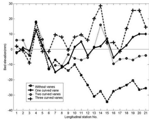
**Fig. 9.** Longitudinal bed profiles 3-cm from outer bank of curved vanes in parallel pattern on 90° bend.
