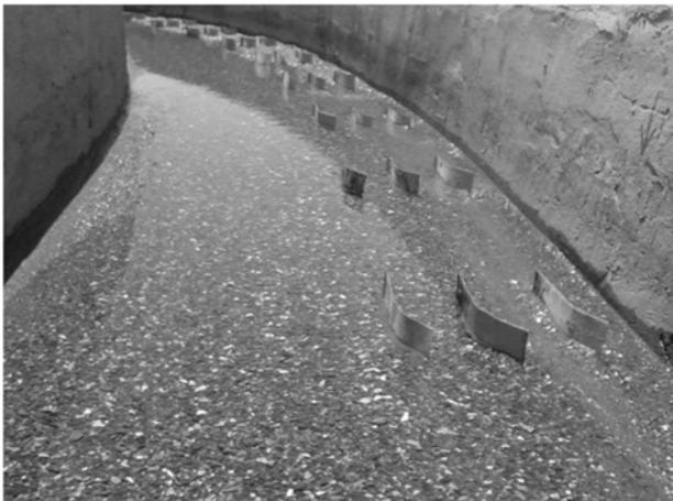
**Fig. 4.** Plan view of curved-vanes installation on the bed of model with 3-vanes in a row at parallel patterns
