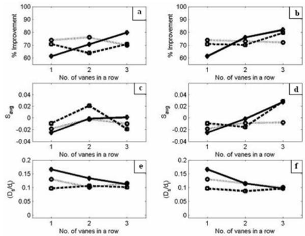
**Fig. 14.** Erosion indices of three shapes of vanes (—●— flat, —◇— curved and ....o.... angled) at different arrays of parallel (a,c,& e) and zigzag (b, d & f) pattern installed at 180o-bend.
