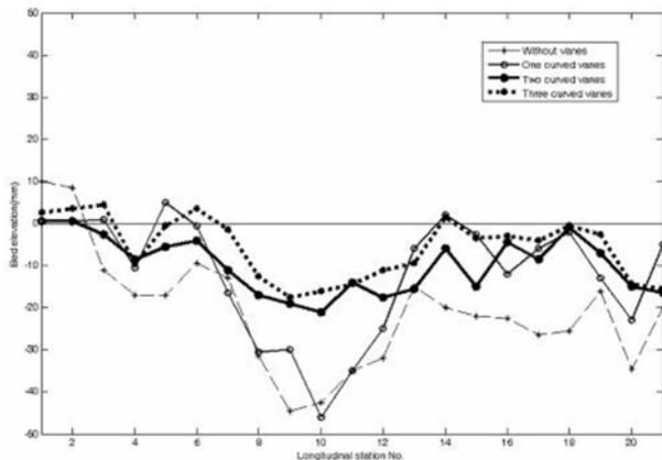
**Fig. 15.** Longitudinal bed profiles 3-cm from outer bank of curved vanes in zigzag pattern on 1800-bend.
