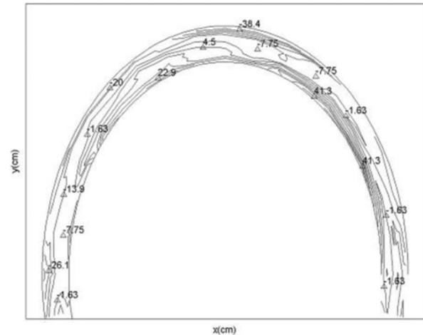
**Fig. 13.** Bed topography of 180o-bend without vanes installation.
