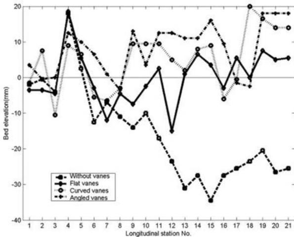
**Fig. 11.** Longitudinal bed profiles 3-cm from outer bank of 3- vanes in a row in zigzag pattern on 90o-bend.
