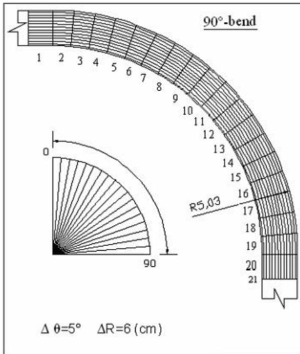
**Fig. 7.** Channel geometry and measured section of 90° bend.
