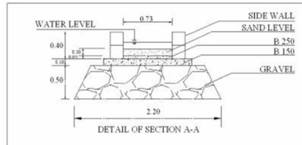
Fig. 2. Details of section A-A.
