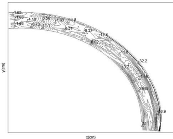
**Fig. 8.** Bed topography of 90° bend without vanes installation.
