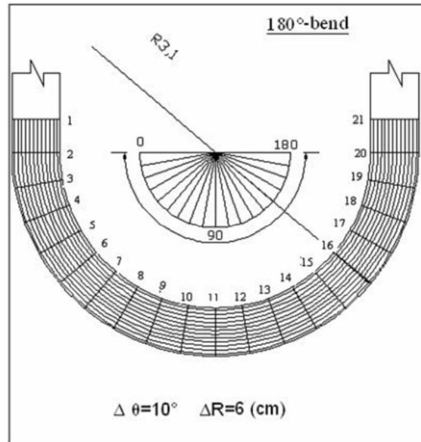
**Fig. 6.** Channel geometry and measured section of 1800 - bend.
