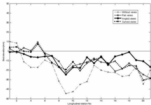
**Fig. 16.** Longitudinal bed profiles 3-cm from outer bank in zigzag pattern on 1800-bend.
