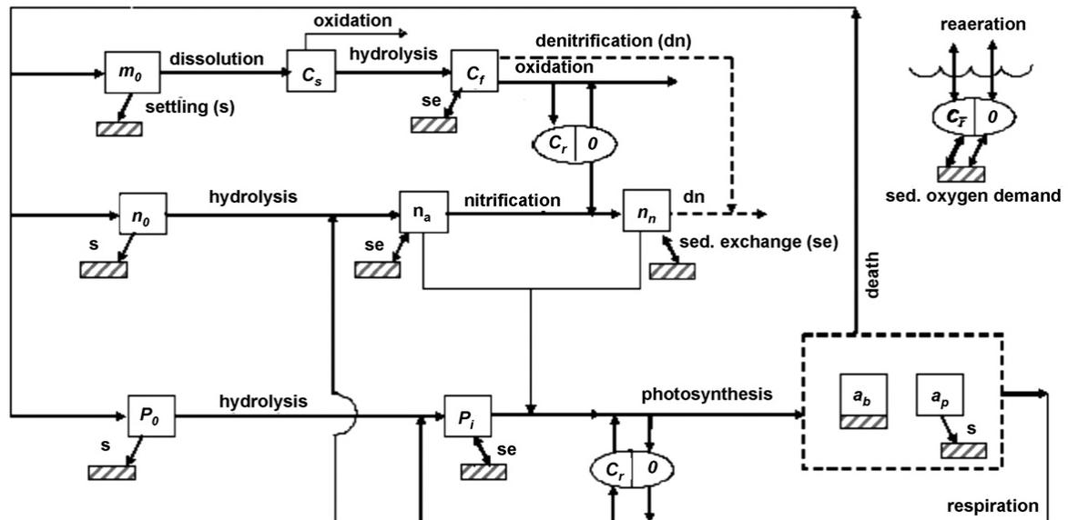
Fig. 3 Schematic diagram of interacting water quality state variables (from Chapra et al., 2006)
