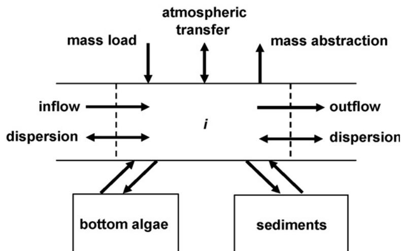
Fig. 2 Mass balance in a reach segment  $i$  (from Chapra et al., 2006)
