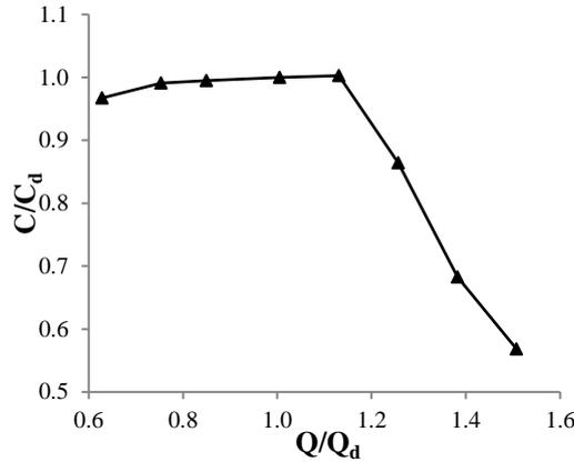
Fig. 6 Discharge coefficients for different discharge
