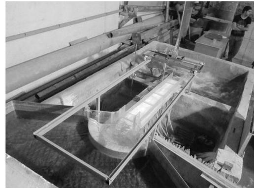
Fig. 4 A view of spillway physical model in scale 1:50
