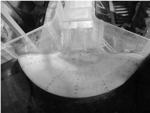
Fig. 3 A view of spillway physical model in scale 1:50
