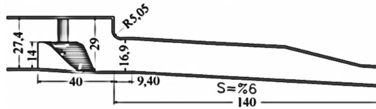
Fig.2 Spillway section (Dimensions in centimeter)
