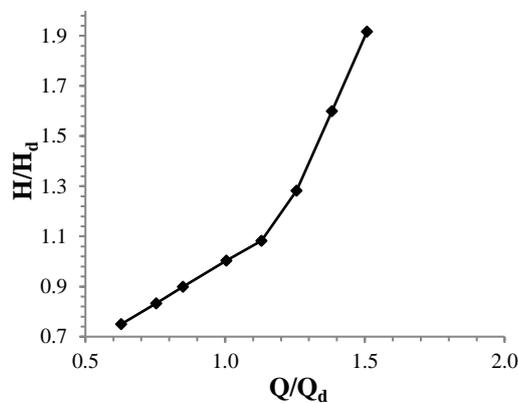
Fig. 5 The variations of head over the spillway crest for different discharge
