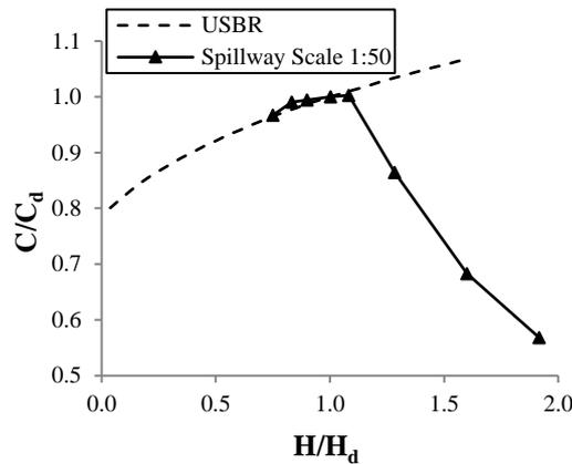
Fig. 7 A comparison of the discharge coefficients for other than the design head
