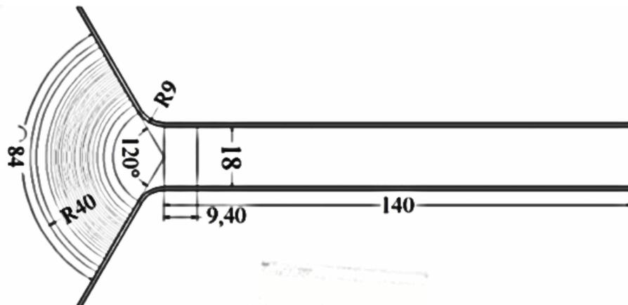
Fig.1 Spillway plan (Dimensions in centimeter)
