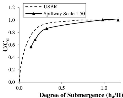
Fig. 8 A comparison of the ratio of discharge coefficients caused by tail water effects
