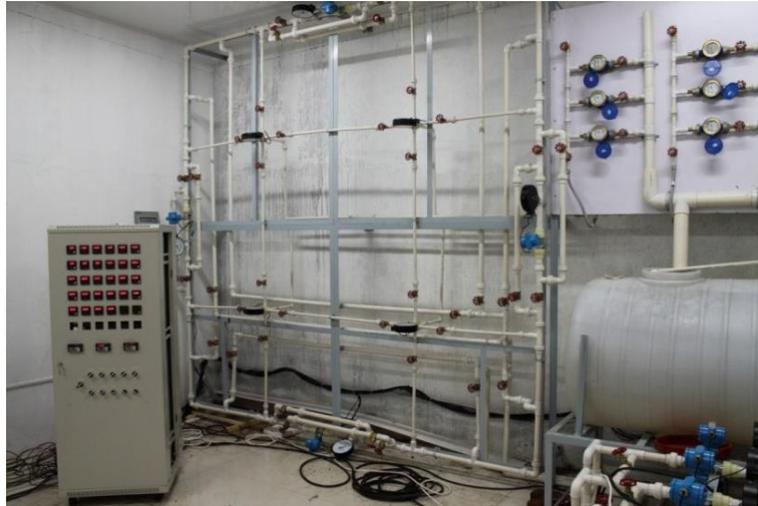
Fig. 2. Experimental platform of Leakage Separation of Water Supply Network
