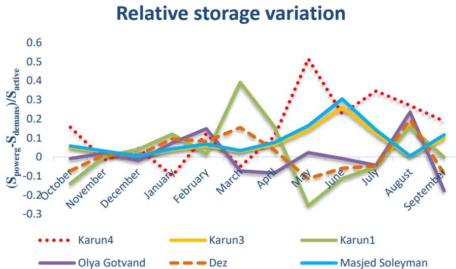
**Fig. 4. The monthly mean values of the reservoir storage volume from the simulation of two different policies**
