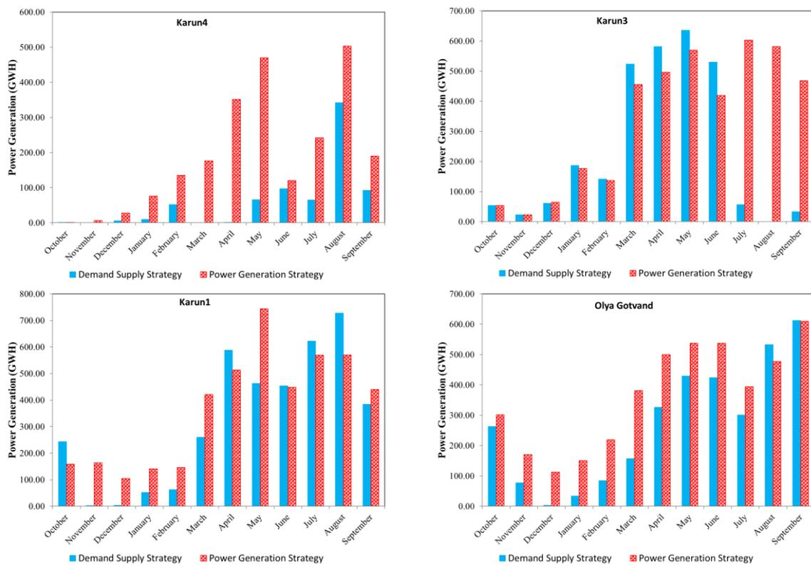
**Fig. 5 - Average monthly power generation in power plants using two different operating policies.**
