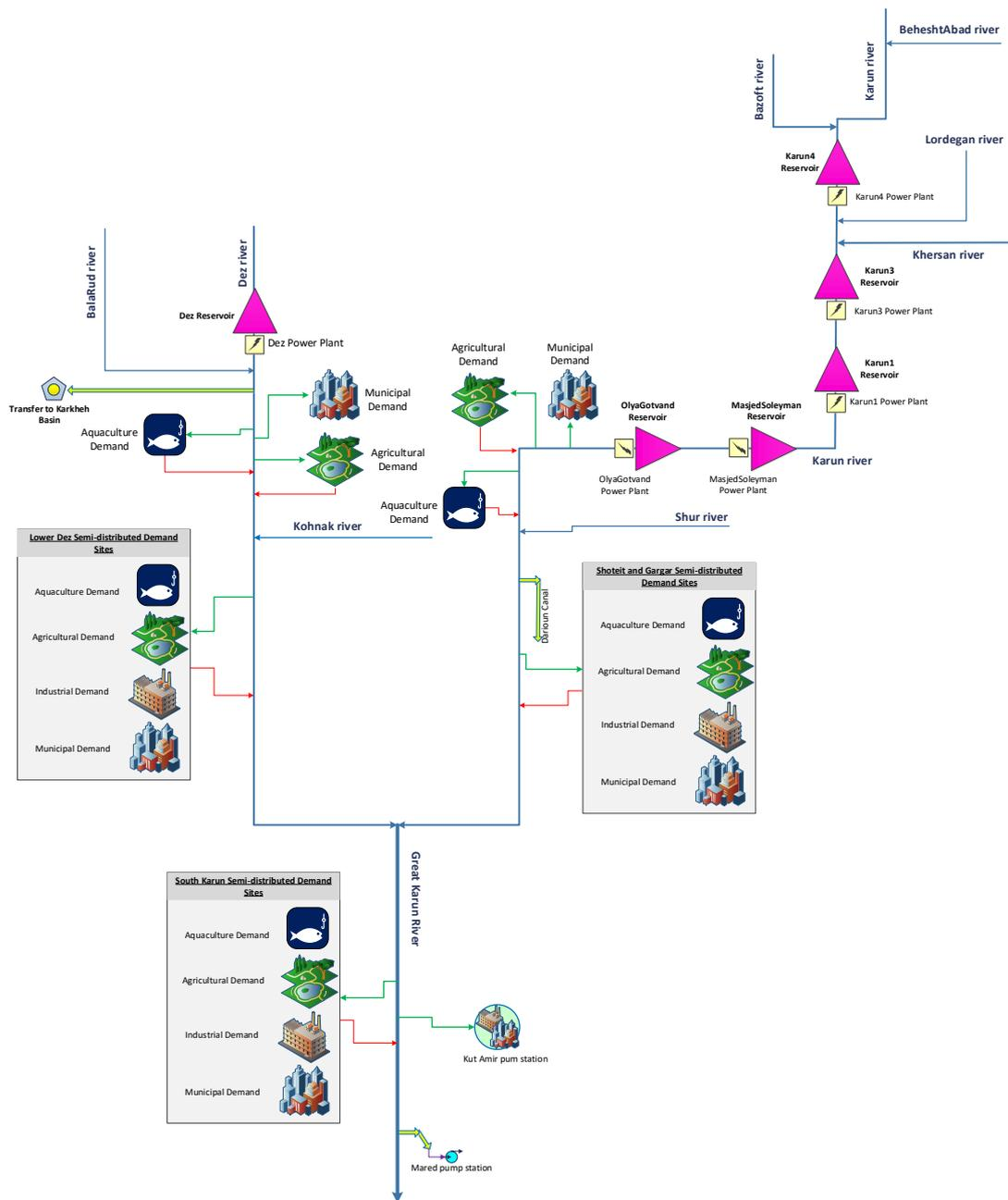
**Fig. 1. The schematic view of the six-reservoir Great Karun River basin**
