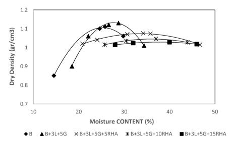
Figure 2. Effect of RHA on compaction curve of the soil stabilized with lime in the presence of sulfate
