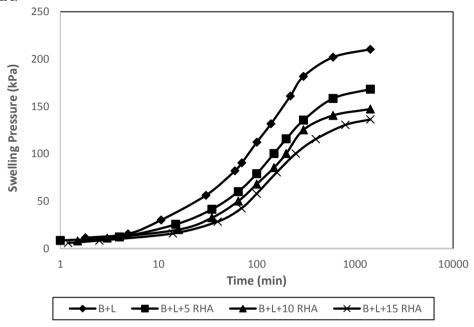
Figure 3. The effect of RHA on swelling pressure of soil stabilized with lime measured immediately after mixing
