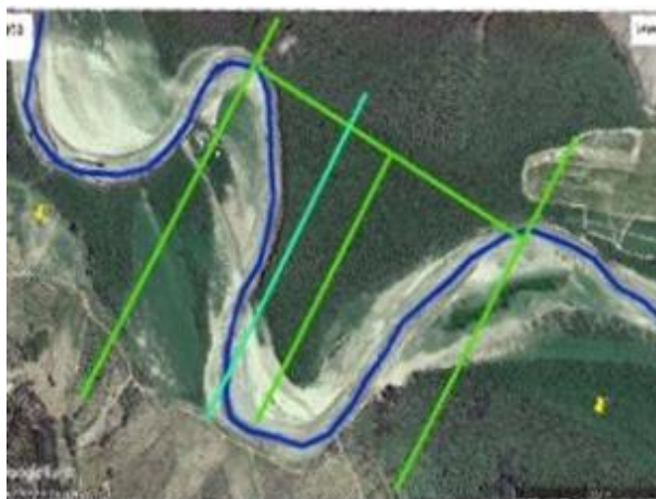
Figure 6. Method of measurement of amplitude, length, and width of meandering
