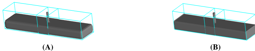
Figure 5. Shows the mesh created in the software for 200 thousand meshes (A) and 600 thousand mesh (B)
