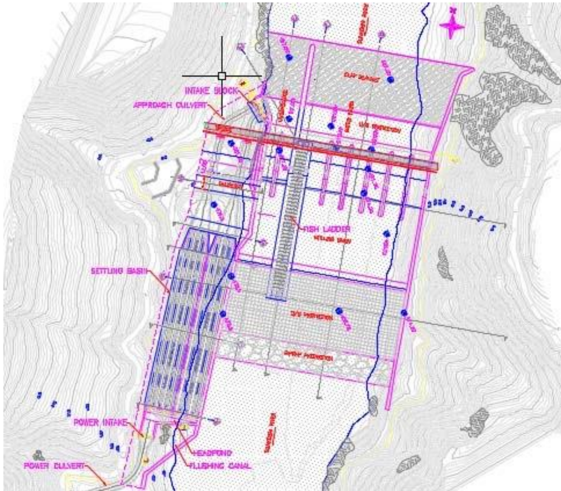
Figure 3. Project layout at head works Area
