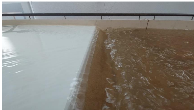
Figure 4. Hydraulic jump formed downstream of GCS
