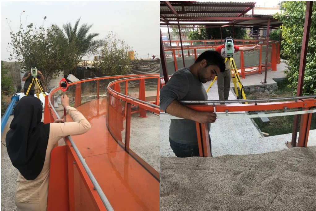
Figure 10. Bend gradation using the Leica Total Station camera
