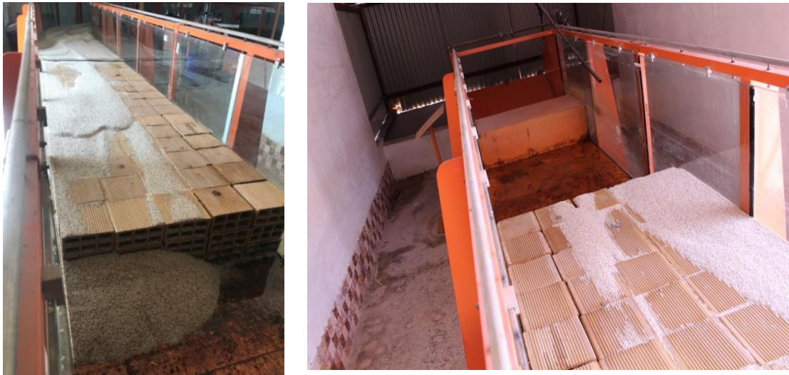
Figure 11. Creating a sediment intake basin at the end of the downstream straight path to prevent sediment from entering the outlet reservoir
