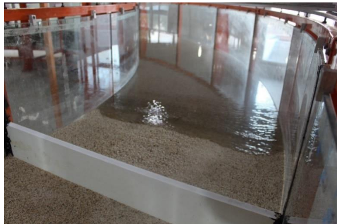
Figure 22. Installation of the sharp-edged spillway in the meandering channel
