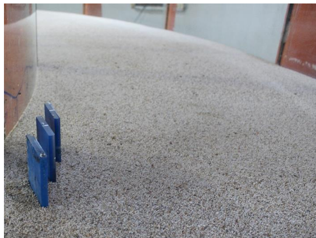
Figure 12. Application of submerged vanes at the outer bend of a meandering channel
