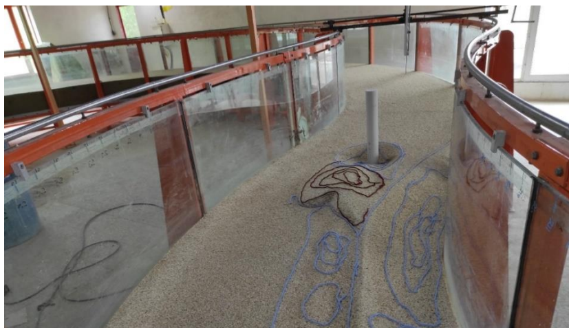
Figure 16. Installation of a cylindrical bridge pier in a laboratory channel and bed variations near it
