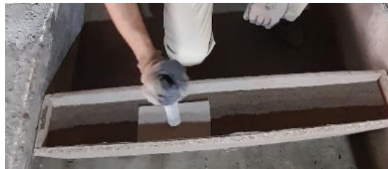
Figure 4. Core compaction in wooden mold
