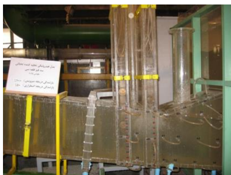
Figure 1. Emergency gate performance of Ghezghaleh Si Dam at 50% openness
