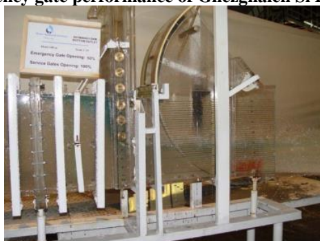
Figure 2. Emergency gate performance of Seymareh Dam at 50% openness
